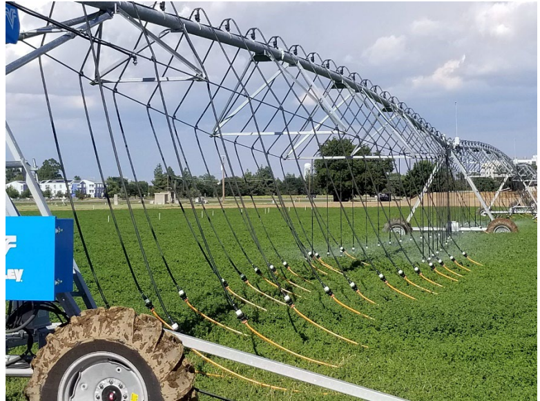
Figure 1. Linear Move Overhead Irrigation System at University of California Davis operating in Alfalfa.
