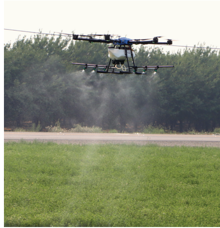
Drones were shown to provide a similar spray coverage as airplanes. Different nozzle types along with speeds and altitudes are being evaluated to achieve maximum performance.
